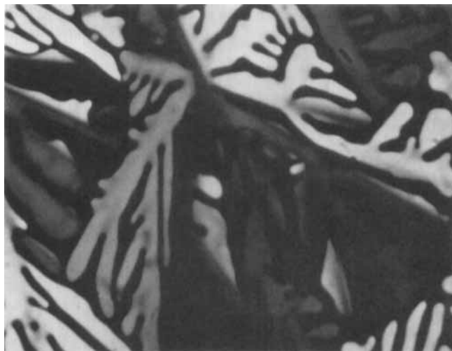
PLATE 1. The separation of the discotic phase from the isotropic liquid for uro-porphyrin I octa-n-dodecyl ester (X100).
